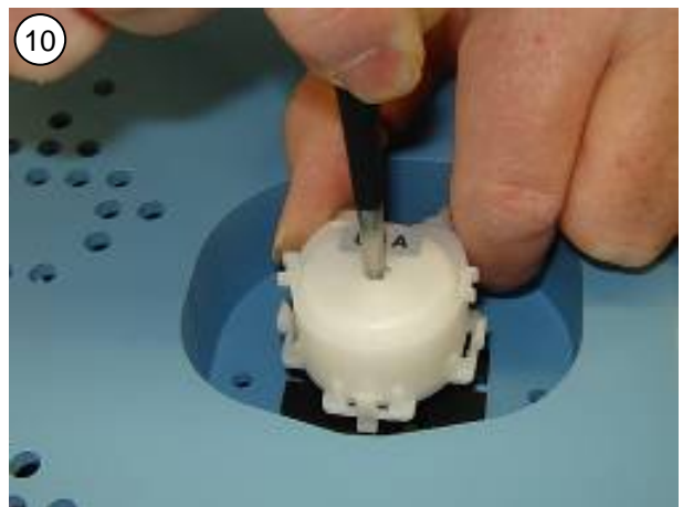
Push the pump cassette on the motor shaft until the snap locks engage. It may be necessary to spread the rollers apart.
